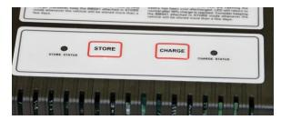
The photo above shows the two operation buttons, and their corresponding LED indicators.
